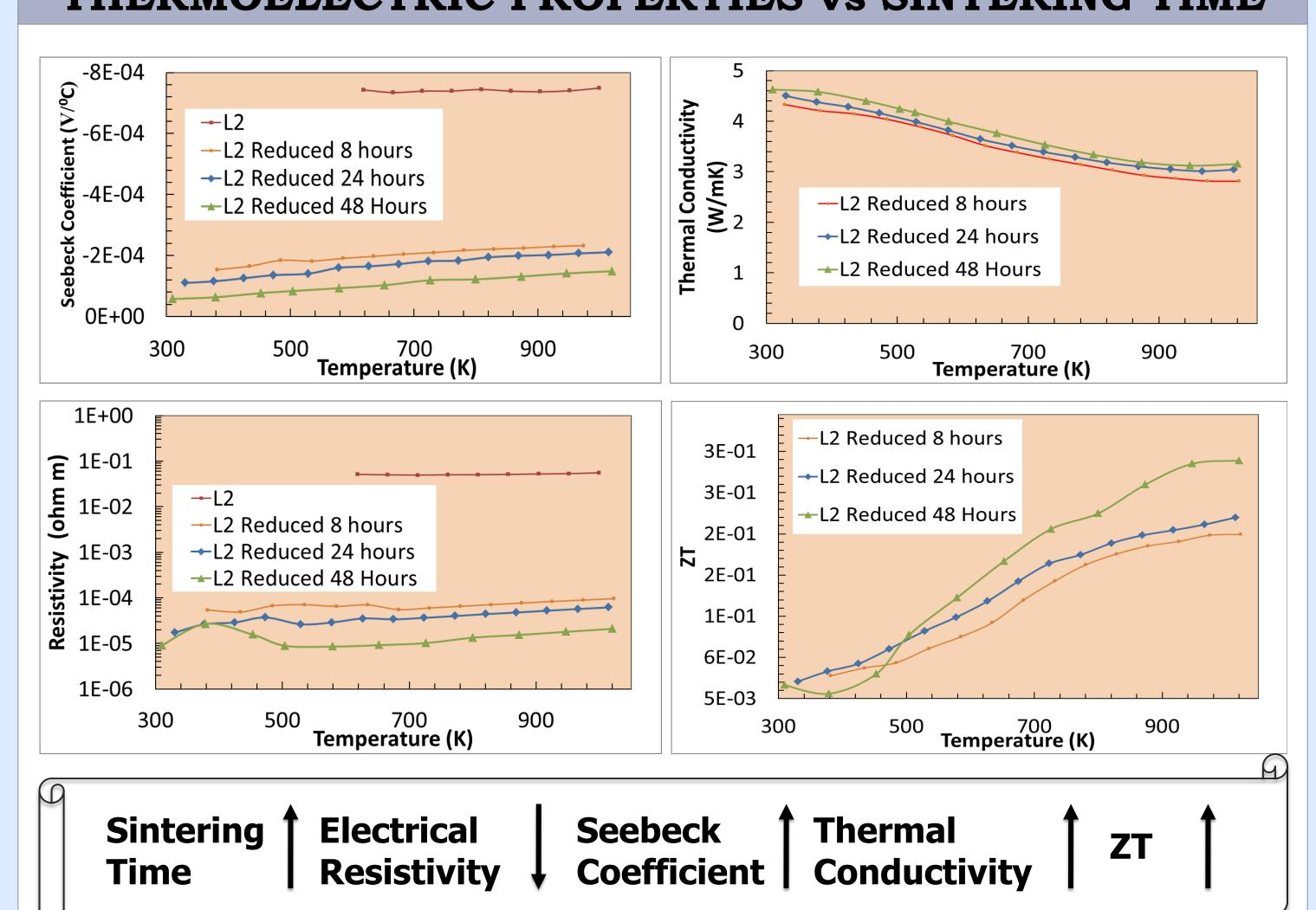
L2 composition was sintered directly in Ar/H2 for different sintering times to study the effect on TE properties as shown above.
