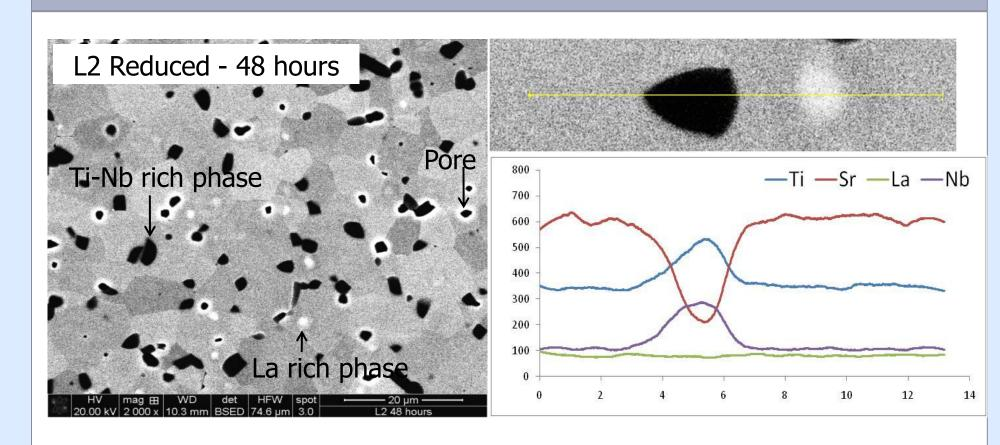
phase increasing EDS on the sintering Line scan microstructure reveals Ti-Nb rich phase and Larich core in the grains. Grain size gradually increases with sintering time.
