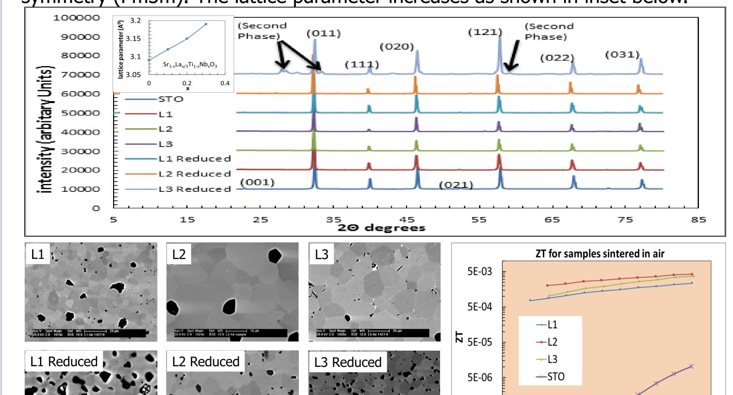
Based on optimum microstructure - crystal structure, improved density and higher TE values among  $\mathbf{x}=0,0.1,\mathbf{0.2},0.3$ ; L2 was selected for further detailed study.
