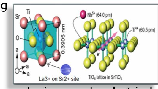
electrical Charge carrier concentration and improved conductivity can be achieved by reduction of Ti<sup>4+</sup> sites to Ti<sup>3+</sup> and creation of oxygen vacancies with normal pressure sintering
